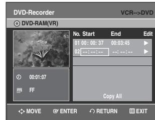
**6** Press the **▲▼** buttons to select desired copylist, then press the **ENTER** or **▶** button.
