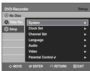
**3** Press the **▲▼** buttons to select **System**, then press the **ENTER** or **▶** button.
