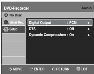
**4** Press the **▲▼** buttons to select the desired audio option, then press the **ENTER** or **▶** button.
