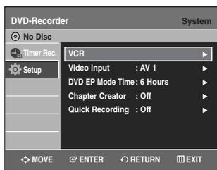
**4** Press the **▲▼** buttons to select **Quick Recording**, then press the **ENTER** or **▶** button.
