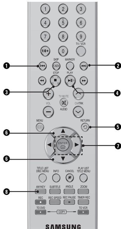
1. **◀◀ button:** Returns to the beginning of the current track when pressed during playback. If pressed again, your DVD Recorder & VCR moves to and plays the previous track. If you press this button within three seconds after playback starts, the previous track will be played. If you press this button after three seconds, the current track will be replayed from the beginning.
