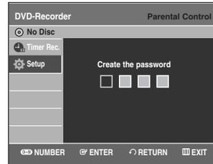
**4** Create a 4-digit password using the 0 to 9 buttons on the remote control.
