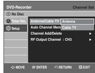
Select the Antenna or Cable TV (Signal Source) that matches the antenna connection you selected on pages 15~17.
