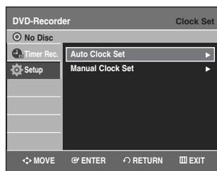
**4** Press the ▲▼ buttons to select **Manual Clock Set**, then press the **ENTER** or ► button.
