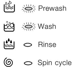
Note: during draining, the LED corresponding to the Spin cycle phase will be turned on.
